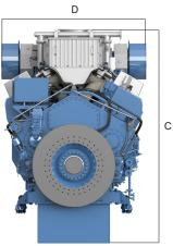
Principal dimensions Cylinder dia. 330 mm. Piston stroke 450 mm. All dimensions in mm.
